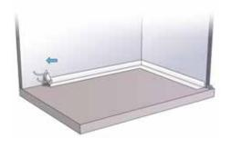
STEP 1: Install TEXFON self-adhesive disconnection band all along the perimeter of the room.
